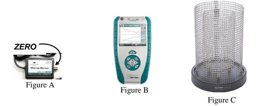
Be sure to zero the charge sensor before every sampling for accurate results. (See Figure A)
