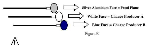
The surfaces of the paddles are soft and easily damaged by misuse --- please take care with them. Also, the black handles of the paddles are easily broken by applying too much pressure.
