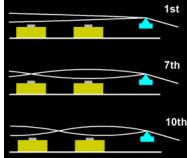
For the seventh harmonic, the pickup on the right is at an antinode, getting a lot of signal, and the pickup on the left is at a node, putting out little signal. When the signals are added together, this harmonic comes across relatively strong.
