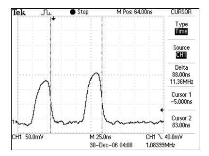
Figure 3: Sample Oscilloscope Screen with far mirror 13.1 meters from beam-splitter. (Note the positions of the vertical cursors and the display of their positions on the screen.)
