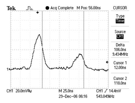
Figure T-1: Sample data for ~16 m separation.
