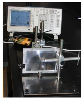
Figure T-2: The oscilloscope and pulse generator w/ the beam-splitter, Fresnel lens, photo detector and laser mounted on the baseplate. (Note: The system works better with the beam-splitter on the other side of the Fresnel lens as described in the lab.)
