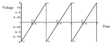
**Figure 2: Graph of Voltage vs. Time for a Sawtooth Wave** (http://www.upscale.utoronto.ca/GeneralInterest/Harrison/Vibrations/transp11.7.gif)
