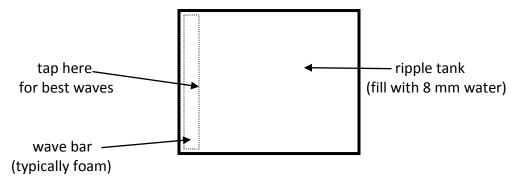
Pour water in the ripple tank so that it is about 8 mm deep. Turn on the light. NOTE: Bulb will get hot!! Do not touch it.
