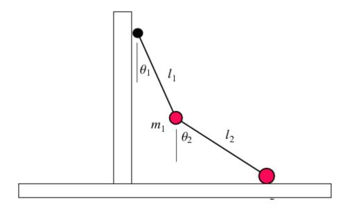
Use the diagram above to indicate the angles of release,  $\theta_1$  and  $\theta_2$ , which are measured with respect to the vertical.
