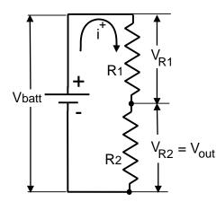
Figure 1. A simple voltage divider. Positive current  $(i^{\dagger})$  flows from the positive pole of the battery through two resistors in series to the negative pole of the battery.
