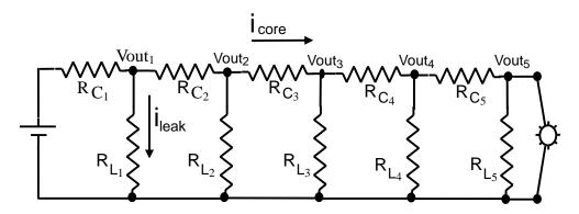
Figure 6: Circuit model for signal losses along a cable.
