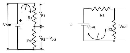
Figure 2: Two equivalent representations of a voltage divider.
