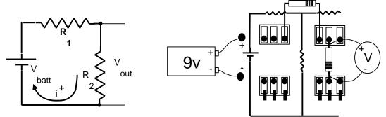
Figure 7. Voltage divider circuit and project board wiring diagram.
