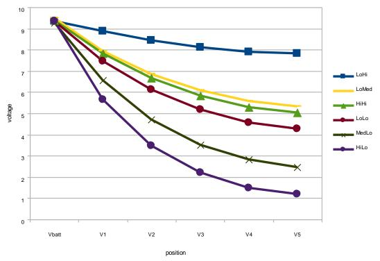
Figure 8: Voltage Divider Data for Different Resistor Combinations. The core resistance is listed first and the leak resistance is listed second.
