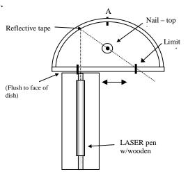
Figure 2: test set-up
